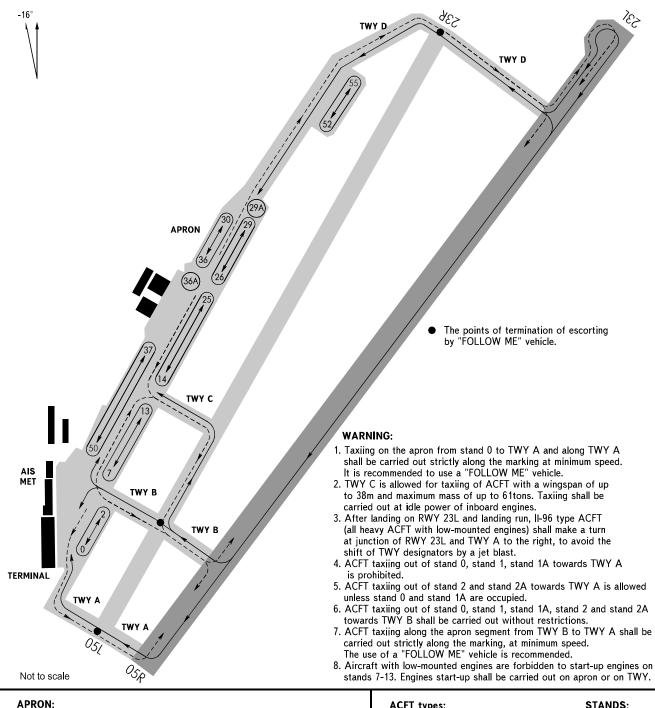
Surface: Asphalt-Concrete Strength: PCN 23/R/B/X/T
