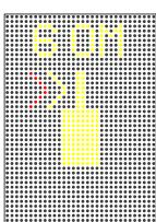
当航空器滑行至距停止线12米(供1-29号机位)/18米(供50-98号机位)处时, 系统显示接近速率信息。When the aircraft is 12m(for stands Nr.1-29)/18m(for stands Nr.50-98) from the stop position, closing rate information is given.
